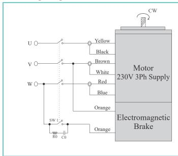
When SW1 is switched ON, Electromagnetic Brake is released & motor starts rotating. When SW1 is switched OFF then Electromagnetic Brake will be applied stopping the motor immediately & holding the load.
